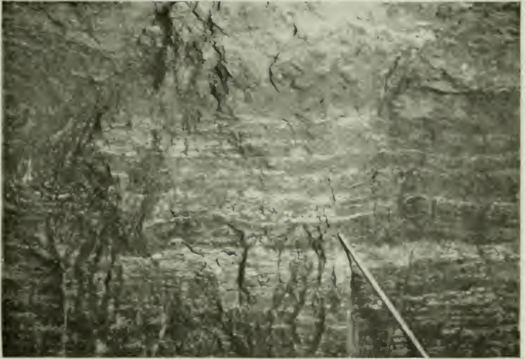
PLATE III.—Face of ore in the No. 2 shoot, Union Mine, near Terry, Black Hills, South Dakota. The original rock is thin-bedded shaly limestone, the ore is silica with small amounts of pyrite and fluorite; gold values about $20. The stratification is here shown preserved in the ore body, although the limestone has been entirely altered to ore. (After U. S. G. S. Prof. paper 26, Plate XVI.) The scale is shown by the shovel handle.
